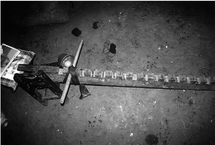
Figure 3.5a The komen or warping frame is ready to begin winding.
